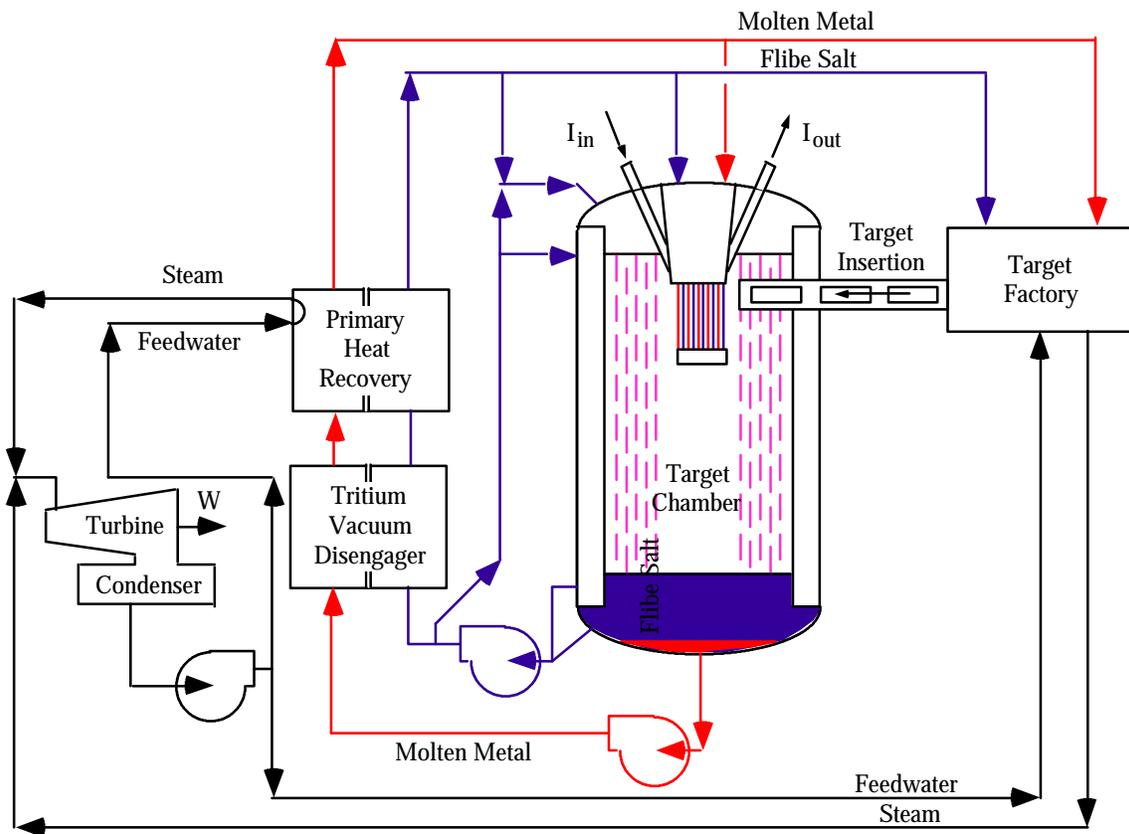
**Fig. II-2.** Schematic flow diagram for the binary-coolant system in a pulsed-power fusion electrical plant.
