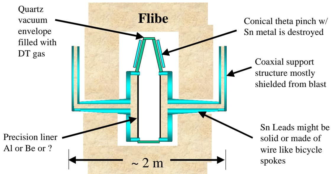
**Fig 2.** Components of MTF target system.
