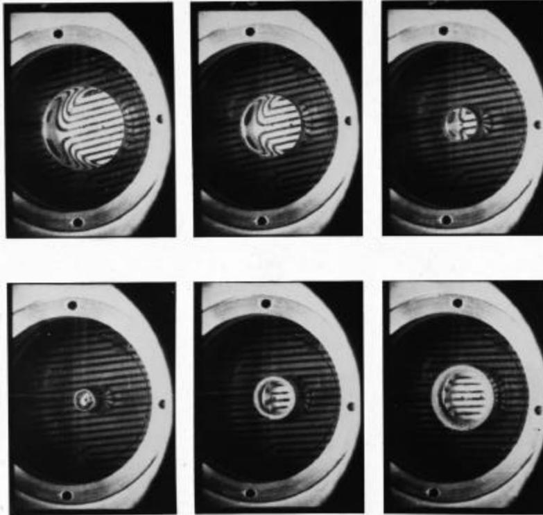
**STABILIZED IMPLOSION DRIVEN BY ANNULAR PISTON**
