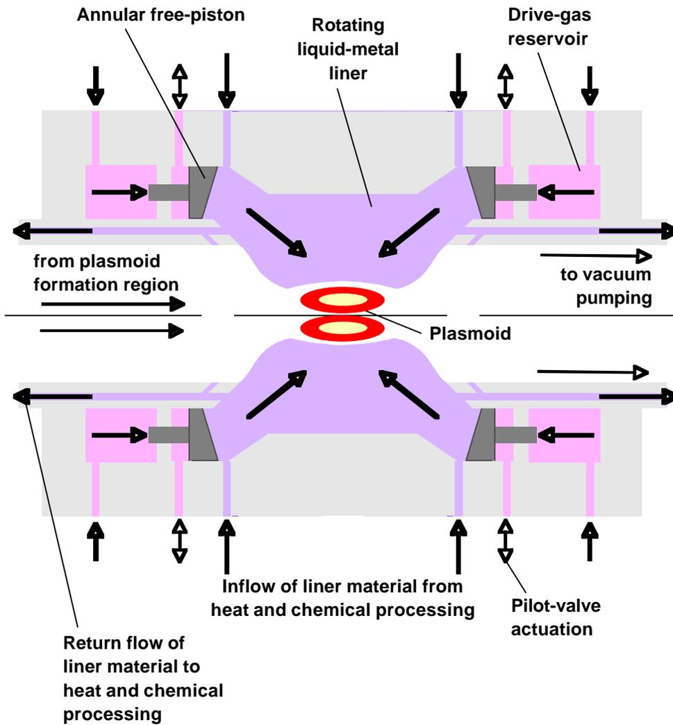
Fig IV2. Schematic arrangement of a LINUS Fusion Power plant
