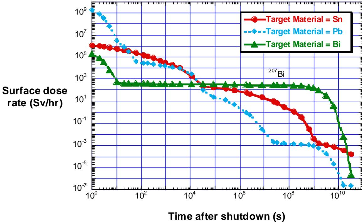
**Fig 3.** Surface dose rate from proposed MTF target materials following 30 years of irradiation at 2500 MW fusion power. Assumes that target materials are recycled on a weekly basis. (Credit J. Latkowski, LLNL)
